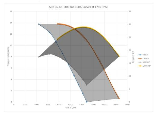
Performance certified is installation Type B: Free inlet, Ducted outlet. Power rating (BHP) does not include transmission losses. Performance ratings do not include the effects of appurtenances (accessories).
